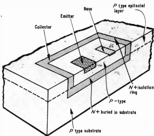
Fig. 1. Cross section view through a CDI transistor
