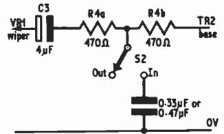
Fig. 9. A tone control circuit is inserted in the position of R4 as shown here with another capacitor
