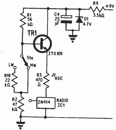
Fig. 5. The integrated circuit is driven from a constant voltage source of 1.3 volts derived from a 9 volt supply
