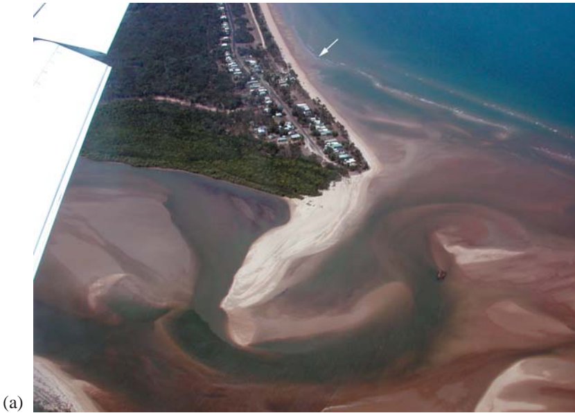
Figure 9: (a) Aerial view of Tully River mouth from above its south bank. The regional direction of coastal transport, under the influence of southeasterly trade winds, is to the north (top left diagonal in the picture). The southerly-directed sand spit which closes much of the mouth has been built by waves that are locally refracted southwards by the presence of nearshore mouth sand bars (cf. Fig. 1c). Storm wave runup in early 2004 was concentrated a few hundred metres north of base of the spit, just north of a protective rip-rap wall, and caused extensive beach and foredune erosion near the point where the Tully offshore mouth bar curves northward to merge into the beach (white arrow).
