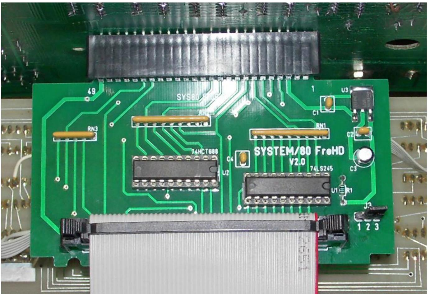
Testing has shown that incorrect power-up sequence may corrupt the FreHD's internal RTC. If you experience any corruption of the RTC change the jumper at J3 to 1-2 else it can be left in the default 2-3 position.
