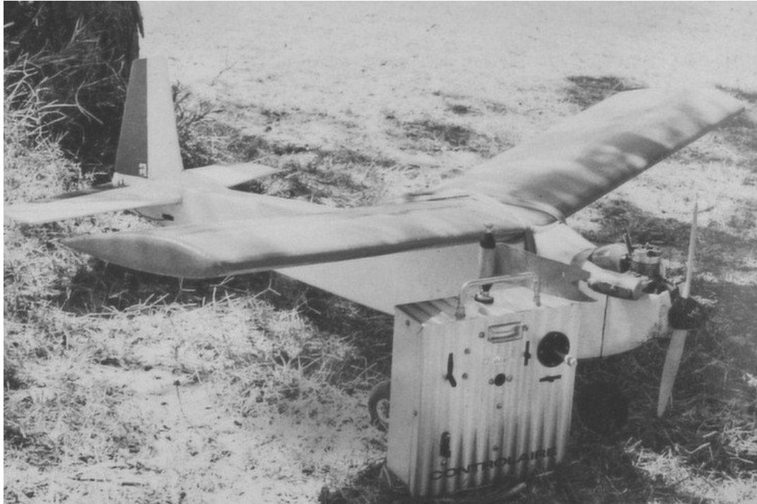
Roland Gee's Aero-Commander from an RCM plan. Enya 19 and Controlaire MAN 234 radio. The pilot described it as being "a beast" to fly. (Courtesy Peter Hardy-Atkins)
