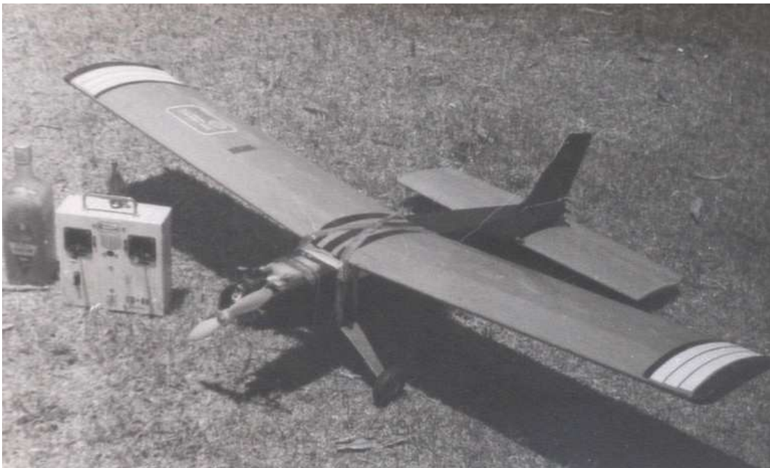
Joe Furfaro's "Rustler" (Reduced Hustler?) was a scaled down Aeroflyte Hustler with reduced dihedral to suit proportional control. Radio and motor are unknown, although carburetor indicates an Enya. (Courtesy Peter Hardy-Atkins)
