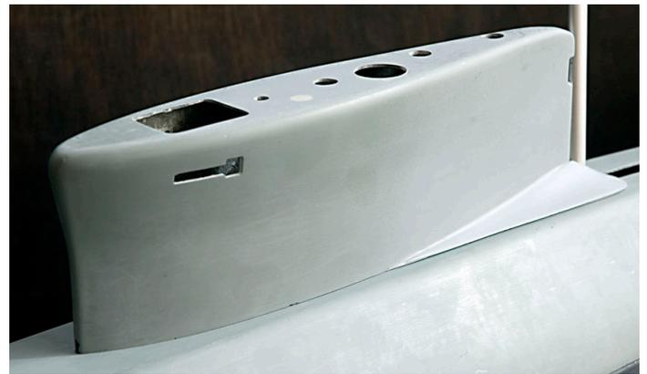
A long narrow aperture on the aft deck provides for the folding snorkel to be retracted. The feature on the starboard side aft of it is a bit of a mystery, but I have concluded it must be the exhaust port for the main diesel engine, to be covered by a maintenance grille. Some of the 200+ free flooding slots in the lower hull are also visible in the photo below.
