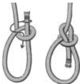
BOWLINE: this knot forms a strong loop that can be easily undone. Some experts can tie this one around their waist using just one hand!
