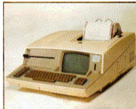
Telex 2000 teleprinter with VDU and memory capability
