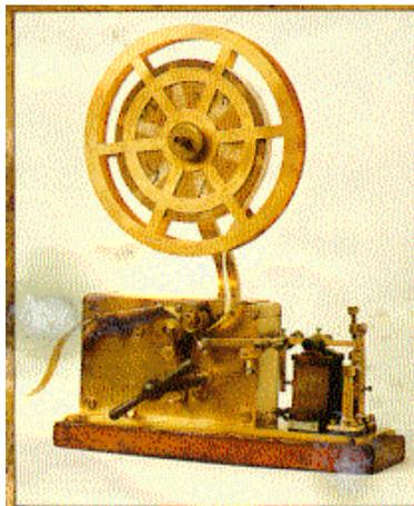
A clockwork driven morse inker from the first days of telegraphy.
