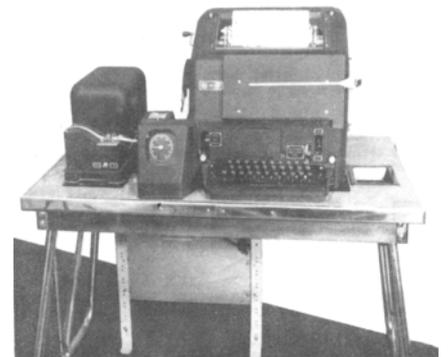
Teletype teleprinter for telex with 5 unit tape facilities
