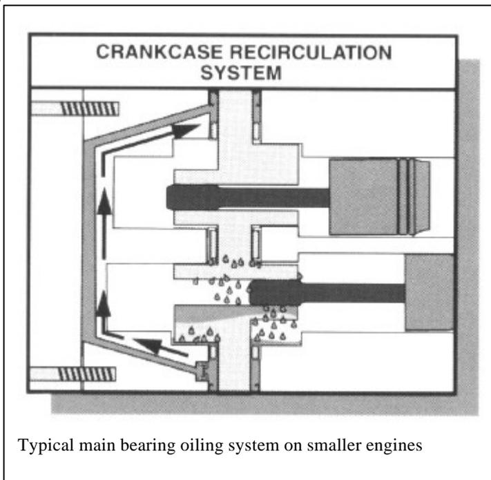
Typical main bearing oiling system on smaller engines
