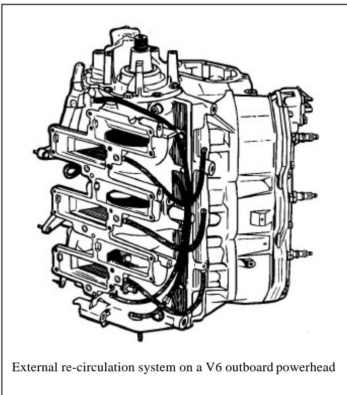
External re-circulation system on a V6 outboard powerhead
