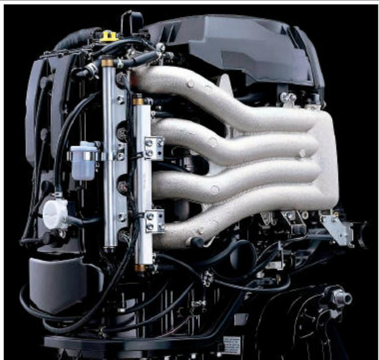
To boost mid range torque, 4-stroke marine engines typically employ very long intake manifold branches, like this 115 HP Johnson outboard. The manifolds must be emptied first.
