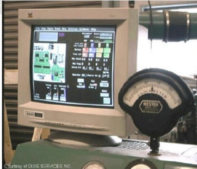
A mixture of old and new. Modern CFR engine control panel showing old style Knock meter alongside computerised control system.
