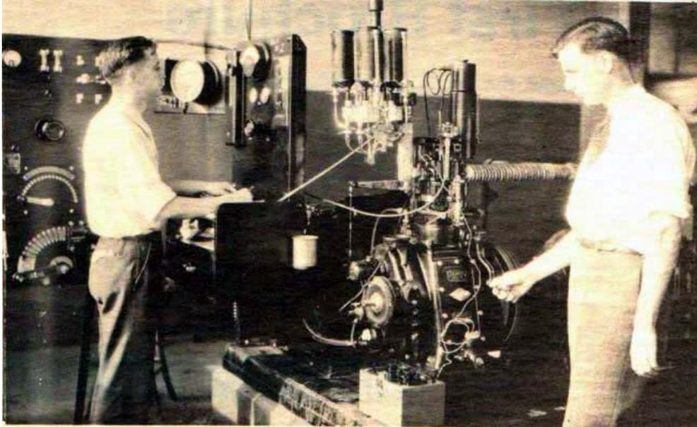
Fuel octane testing in the 1930's. Operator on the left is observing the knockmeter (centre, top of panel) while operator at right is gripping the handle that moves the cylinder up and down to vary compression ratio.
