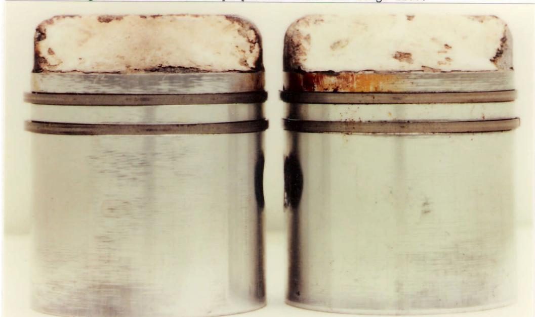
Comparative testing – 50 hours at wide open throttle and 4500 rpm.
