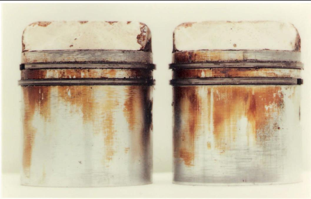
ABOVE: With ordinary two-stroke oil, the pistons are heavily coated and the rings are partly stuck.
