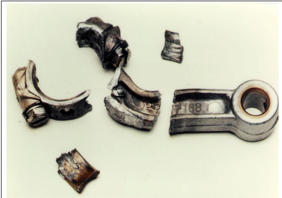
The results of an oil that failed the lubricity test! One melted aluminium con-rod.
