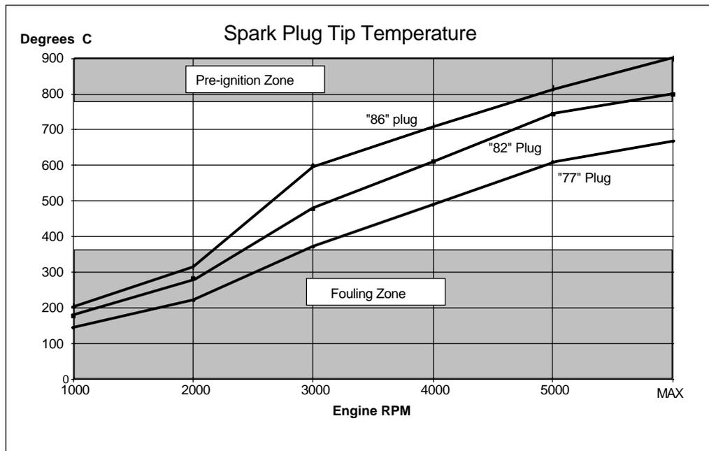
Figure 2 - Results of thermocouple spark plug tests on a large outboard.
