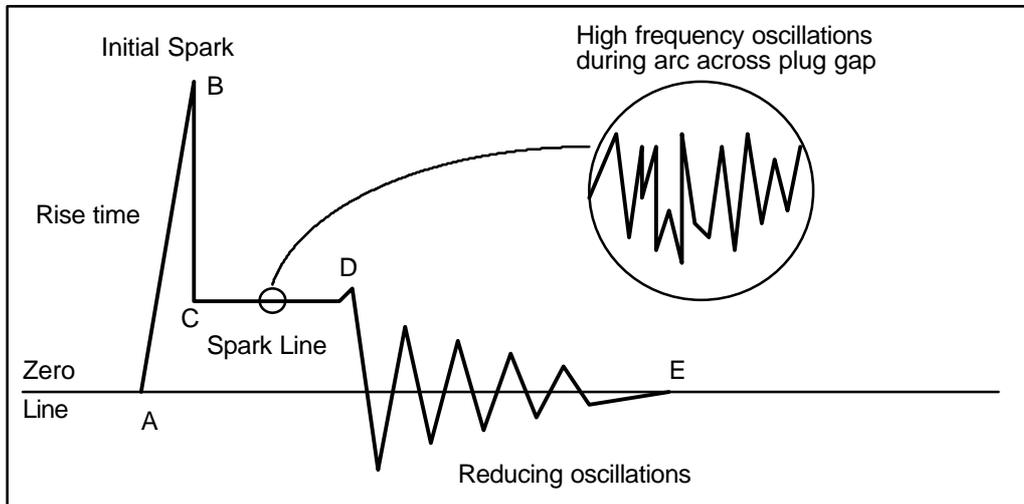
Figure 6 - Oscilloscope trace of ignition secondary voltage.
