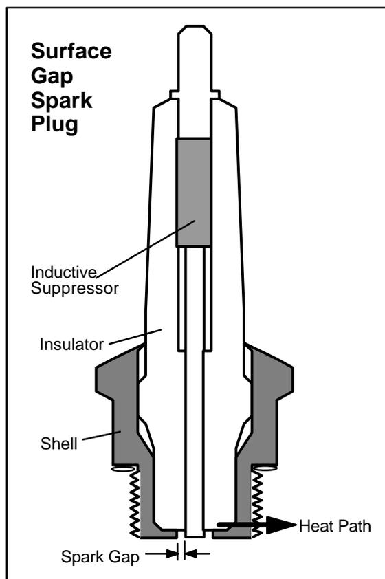
Figure 4 - Construction of a surface gap spark plug.
