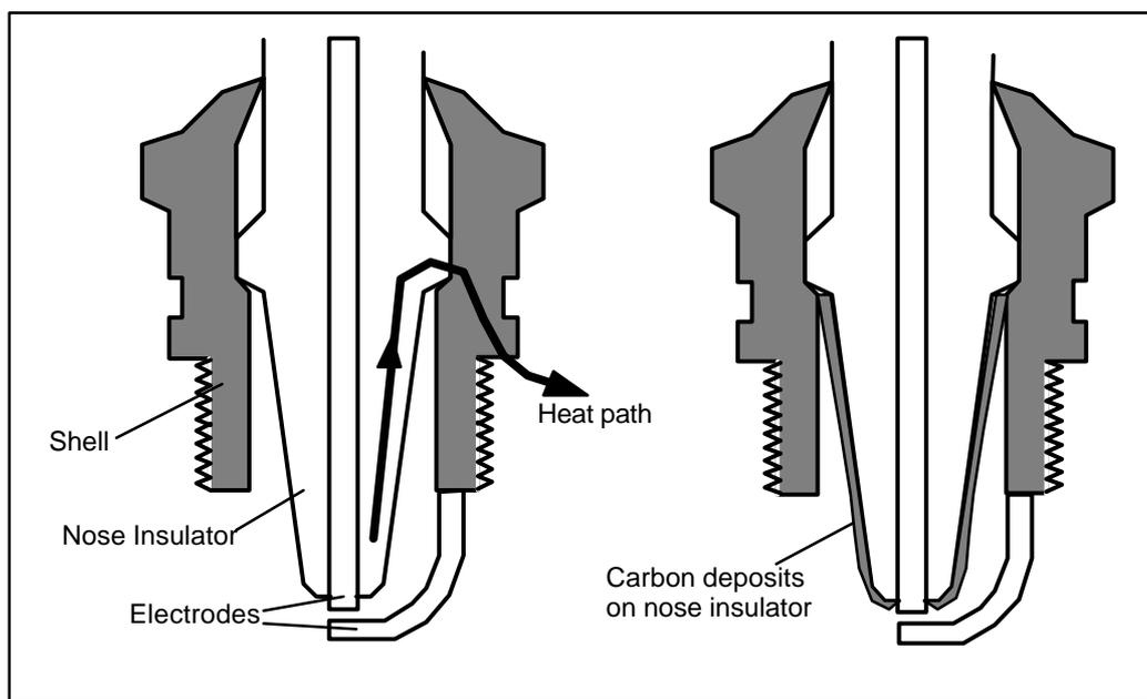
Figure 1 - Firing end of a typical spark plug.
