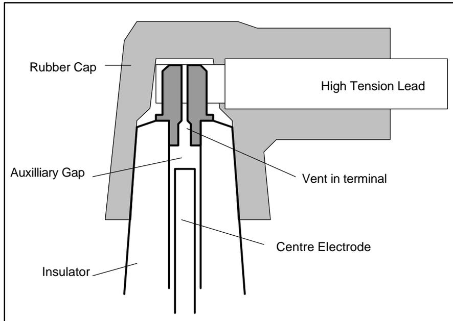
Figure 5 - Location of the auxiliary gap and gas vent.
