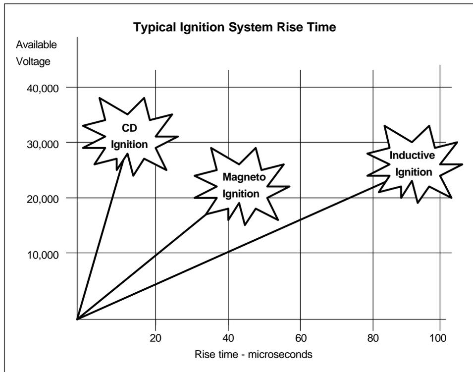
Figure 3. - Rise time comparison between different ignition system types.
