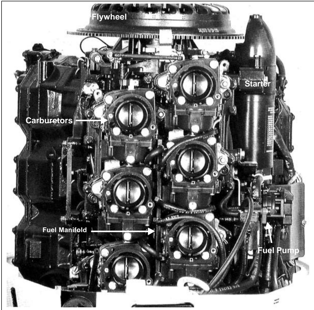
The business end of a 3 litre, 90 degree V6, 250 HP outboard fuel system, with the air silencer removed.
