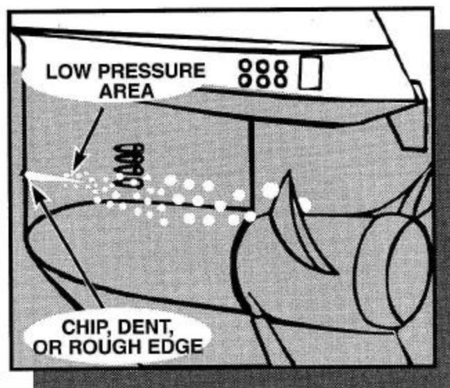
Figure 4 - How damaged leading edges on the gearcase can cause propeller cavitation.
