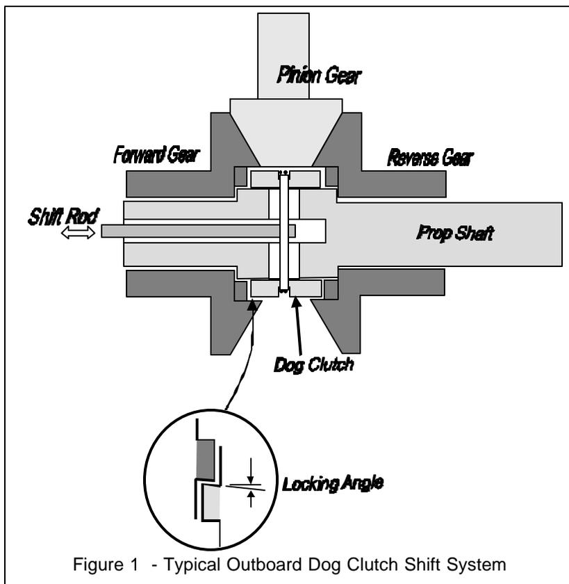
1. Always shift at the lowest possible speed, engine at idle and boat stationary. A low engine idle speed is very important here.
