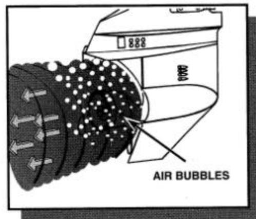
Figure 6 - Propeller ventilation
