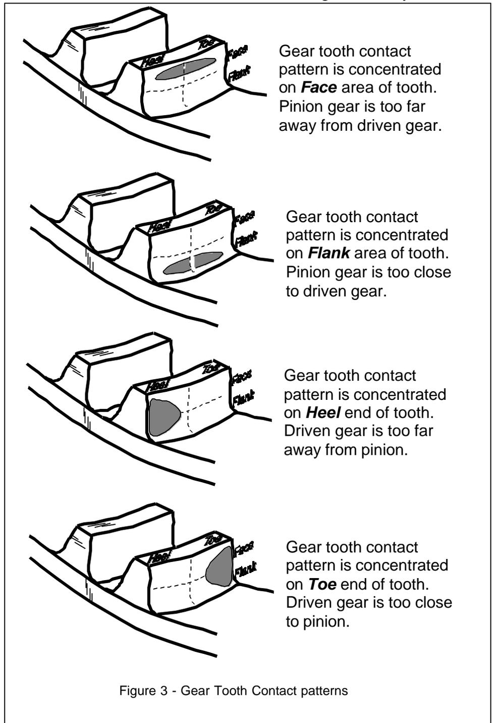
Gear tooth contact pattern is concentrated on **Face** area of tooth. Pinion gear is too far away from driven gear.
