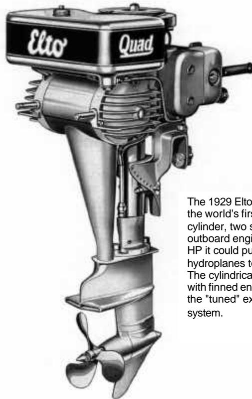
The 1929 Elto Quad was the world's first 4 cylinder, two stroke outboard engine. At 18 HP it could push racing hydroplanes to 45 mph. The cylindrical chamber with finned end caps was the "tuned" exhaust system.
