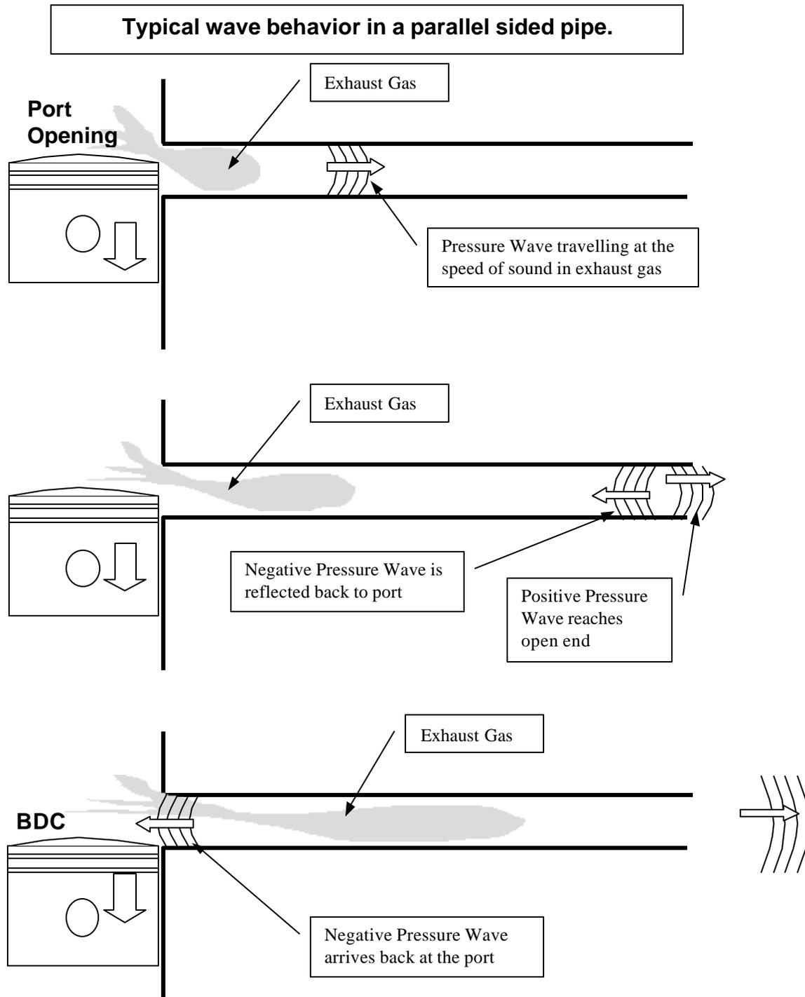
The breakthrough was in understanding how pressure waves, or sound waves, travel along the exhaust pipe and can change the pressure in the system. When the exhaust port opens the still quite high pressure in the cylinder causes a positive pressure wave to travel along the pipe, at the speed of sound. When it reaches the open end of the pipe
