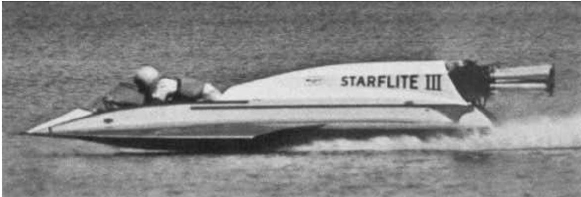
An example of this type of system is shown in the picture of Starflite III a hydroplane that set the worlds outboard speed record at 123 MPH (198 KPH) back in 1960. The V4 1.5 litre two-stroke engine was based on the Evinrude 75 HP outboard motor of the day and produced about 120 HP. The exhaust system used 4 megaphones and is bigger than the engine. Noisy but very effective.
