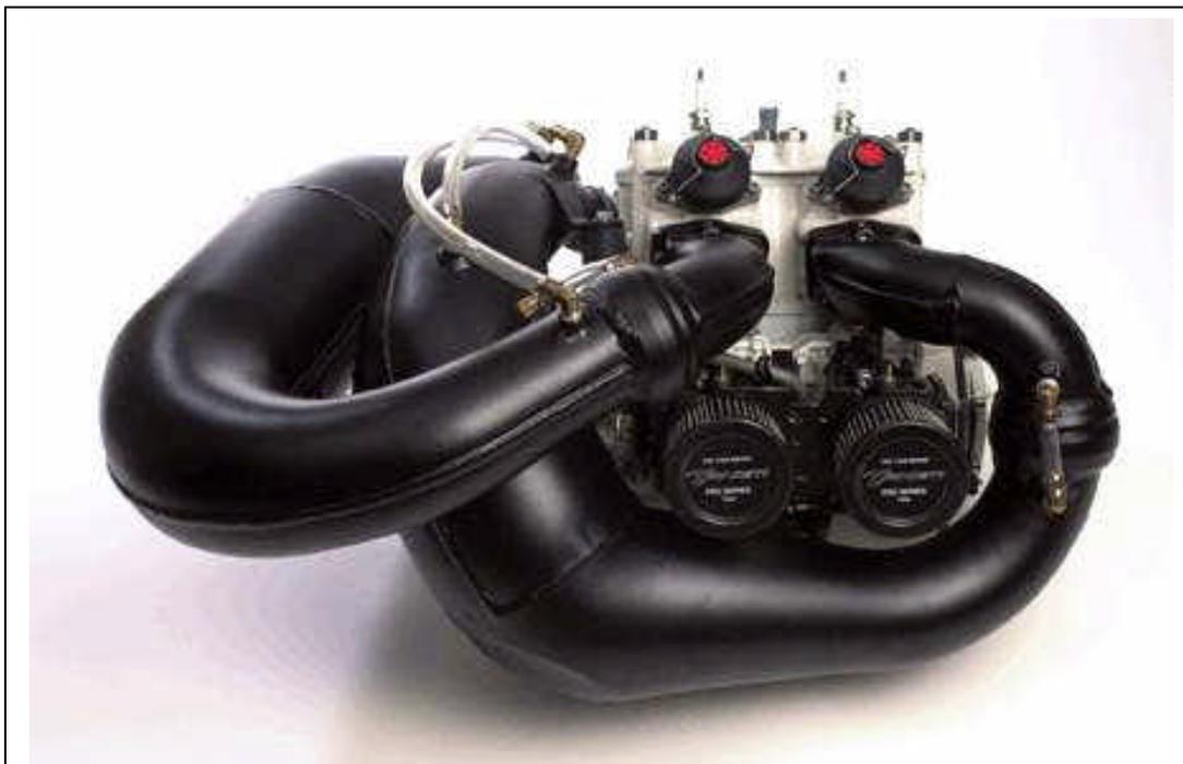
Twin expansion chambers fitted to a twin cylinder 950 cc Seadoo Rotax engine, by US speed equipment maker Factory Pipe. The pipes are water jacketed and water injected by an electronic controller to vary the gas temperature and get the sonic waves to arrive at the right time over a wider RPM range. Engines with this setup can produce over 160 HP (120 kW).
